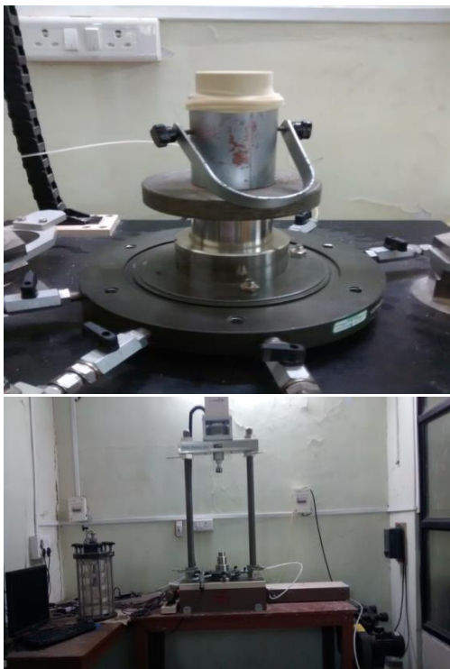
Fig.1. Cyclic triaxial Test Apparatus and sample preparation.
