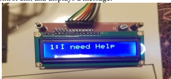
Fig.11: LCD showing emergency message
