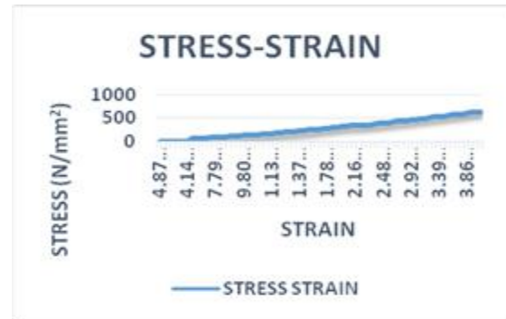
Fig 15. Stress strain curve of hexagonal wide opening
