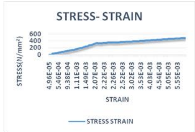
Fig 14. Stress strain curve of hexagonal opening 25 mm
