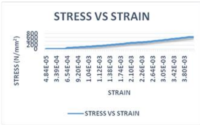
Fig17. Stress strain curve of rectangular opening 25mm
