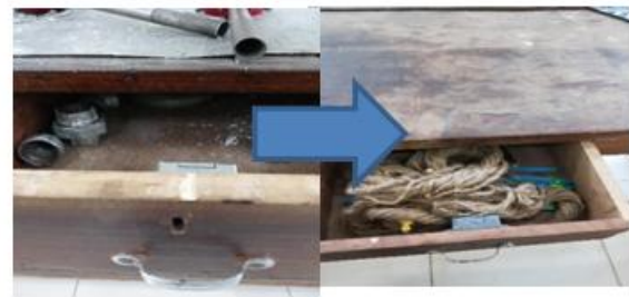
Fig 5.2 - This shows us the implementation of the 2nd step in 5S that is Set in Order which is the practice of sequentially storage the right item, right time , right place can be picked effectively and efficiently and easy to access for everyone.
