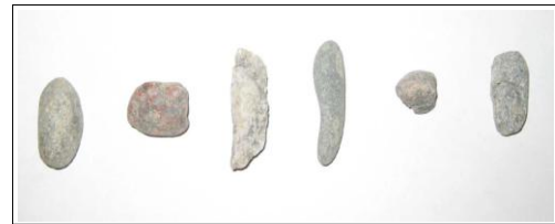
Figure 3.4: Different shapes and sizes of aggregate passing the 16 mm sieve, originating from the same quarry
