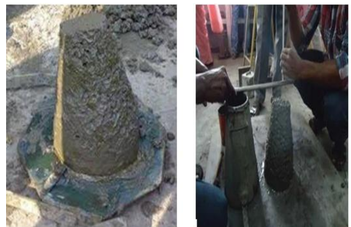
Figure 2 Slump test on fresh concrete
