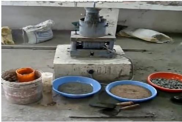
Fig 3 Vee-bee consistometer test on fresh concrete
