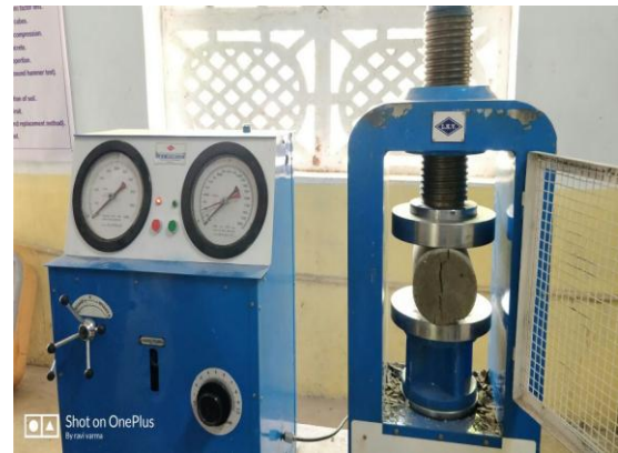
Fig:3.1 Split tensile strength testing
