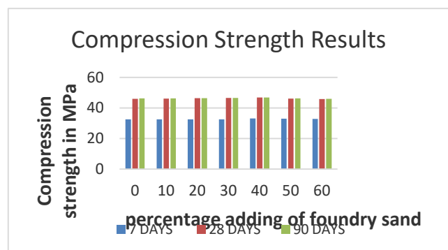
Fig 4.4: variation of compressive strength of aluminium slag (25%) added concrete on partial replacement of fine aggregate with foundry sand at 7 days, 28 days and 90 days
