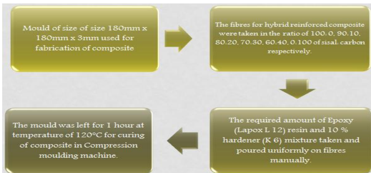
Fig 2 Mould and compound specimen preparation[42-44]
