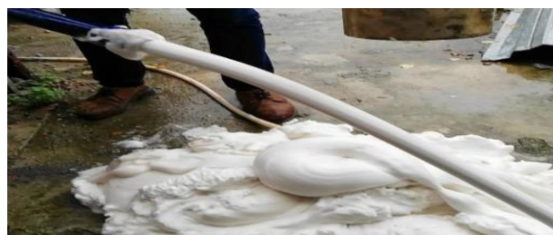
Fig. 1 Foam production from Portafoam PM 1
