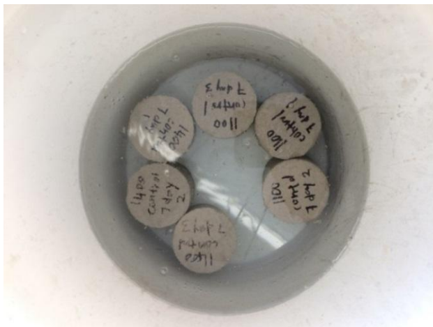
Fig. 3 Water absorption test of foamed concrete specimens
