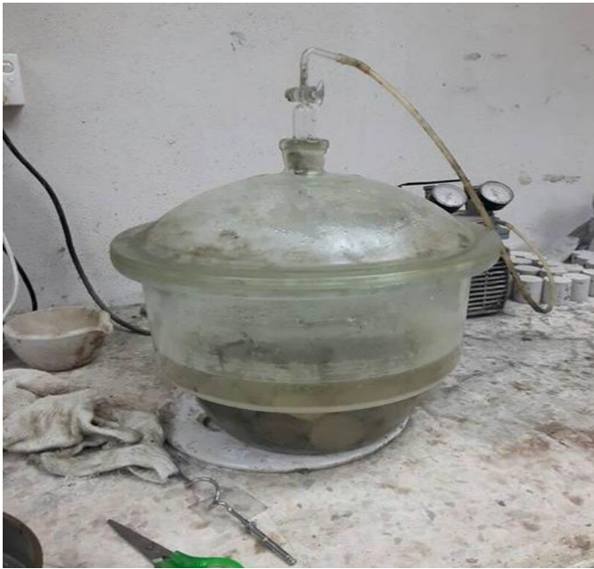
Fig. 4 Foamed concrete specimens in a desiccator under vacuum
