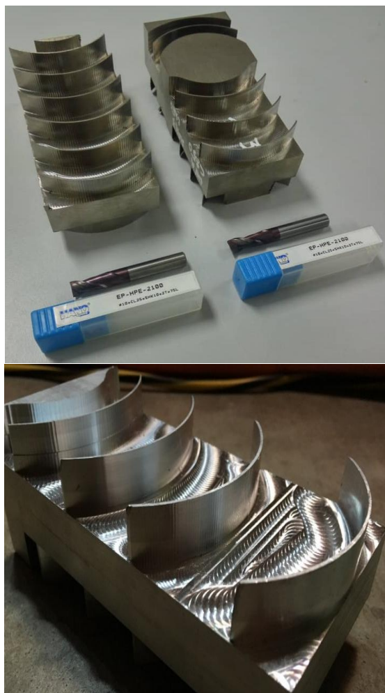
Fig. 2 Completed machined part by 3 axis CNC milling machine
