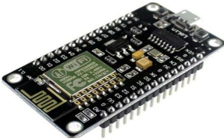
**Fig4:ESP -12E based NODEMCU**
