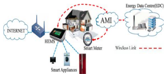
Fig. 7. Smart Metering System with 5G network
