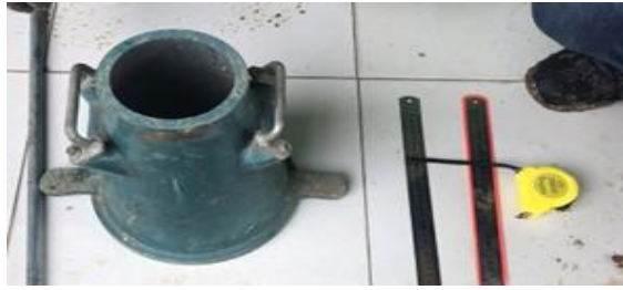
Fig. 4. Slump test equipment
