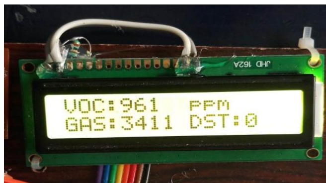
Fig 5.2.4 Exceeded level of MQ 2 sensor gases in air
