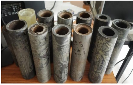
Fig.2: Prepared FGNNFE cylinder specimens.
