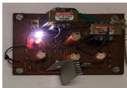
Fig.19. Power Supply Circuit
