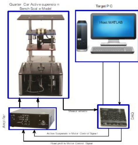
Fig.5 . Block diagram of hardware setup
