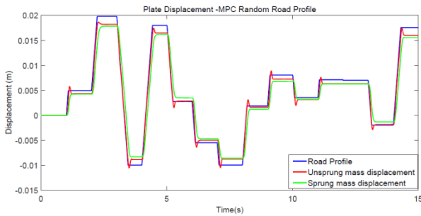
Fig.10. Unsprung and sprung mass motion for random road profile (MPC)
