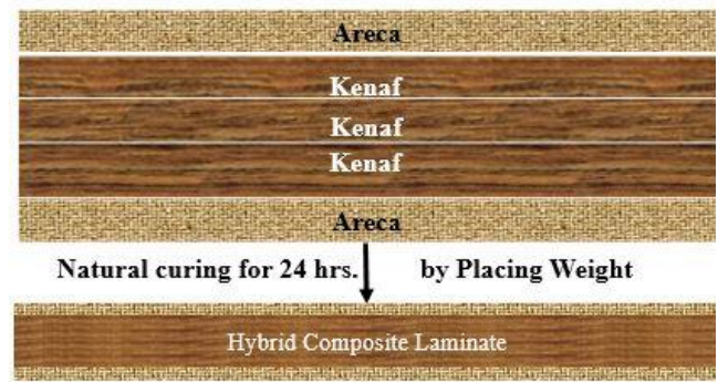
Fig.1 Fabrication of the hybrid composite
