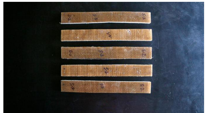
Fig.2 Tensile specimen of the hybrid composite
