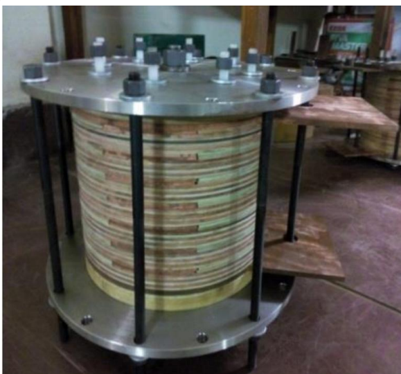
Fig.12 Bitter Coil of 24 \mu\text{H} at 400 Hz. This has 8 m \Omega DC resistance and weight of 68 kg
