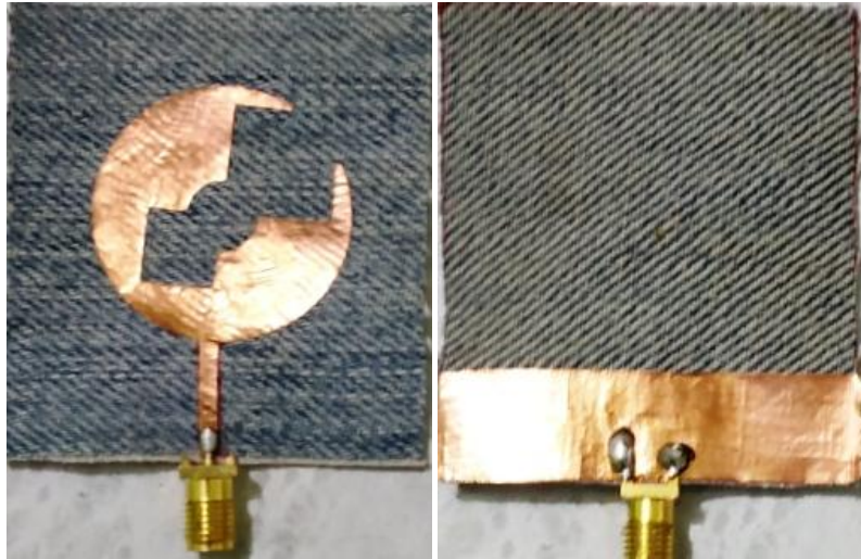
Figure1. 8: Proposed Antenna after fabrication process (i) Front View (ii) Back View.
