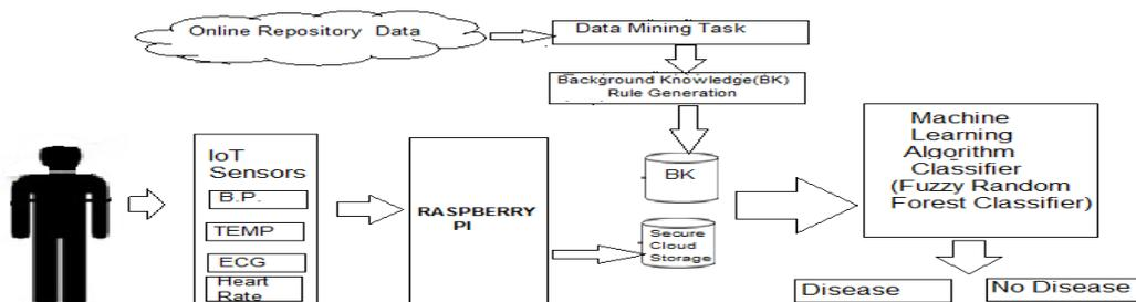
Figure 1: System Architecture
