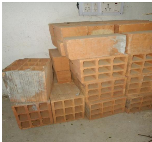
Fig 1: Samples of hollow bricks used for construction of biomass dryer firing chamber
