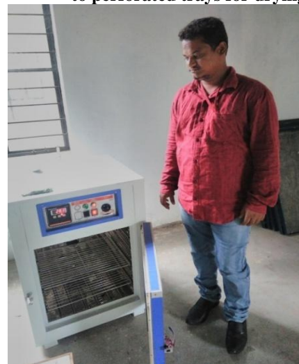
Figure 3: Conducting moisture drying experiment in a hot air oven till equilibrium.
