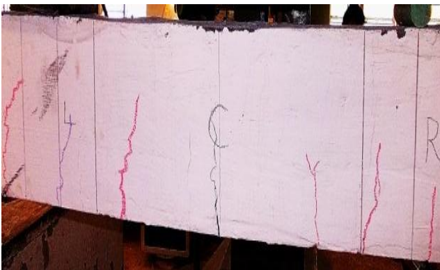
Fig 12 Failure pattern of GP0+BA0 (RC beam)
