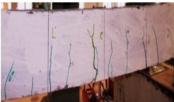
Fig 12 Failure pattern of GP10+BA10 (RCW beam)
