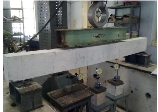
Fig 1 Loading arrangement of RC beam
