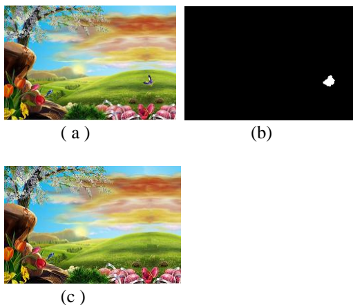
Fig. 2 Object Removal by LB Method (a) the input image. (b) the mask prepared to remove the object (c) the inpainted image after removal of object.
