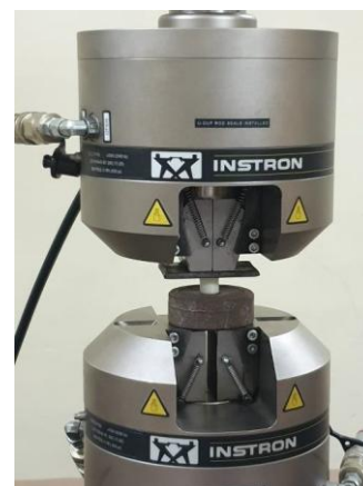
Fig 6 Compression test on Instron 8801 universal loading machine
