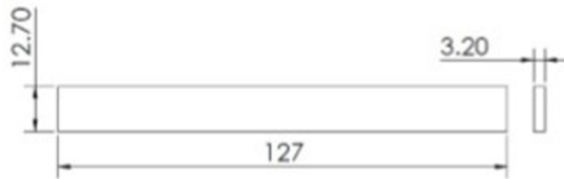
Fig 7. Bending Test Specimen Dimensions (In Mm)
