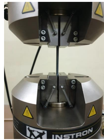
Fig 4. Tensile Test On Instron 8801 Universal Loading Machine
