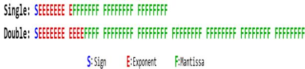
Fig 3. IEEE 754 standard floating-point memory allocation
