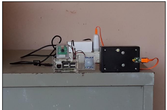
Fig. 4 The installation of sensor and equipment with Raspberry Pi Model B+ board in front of the house
