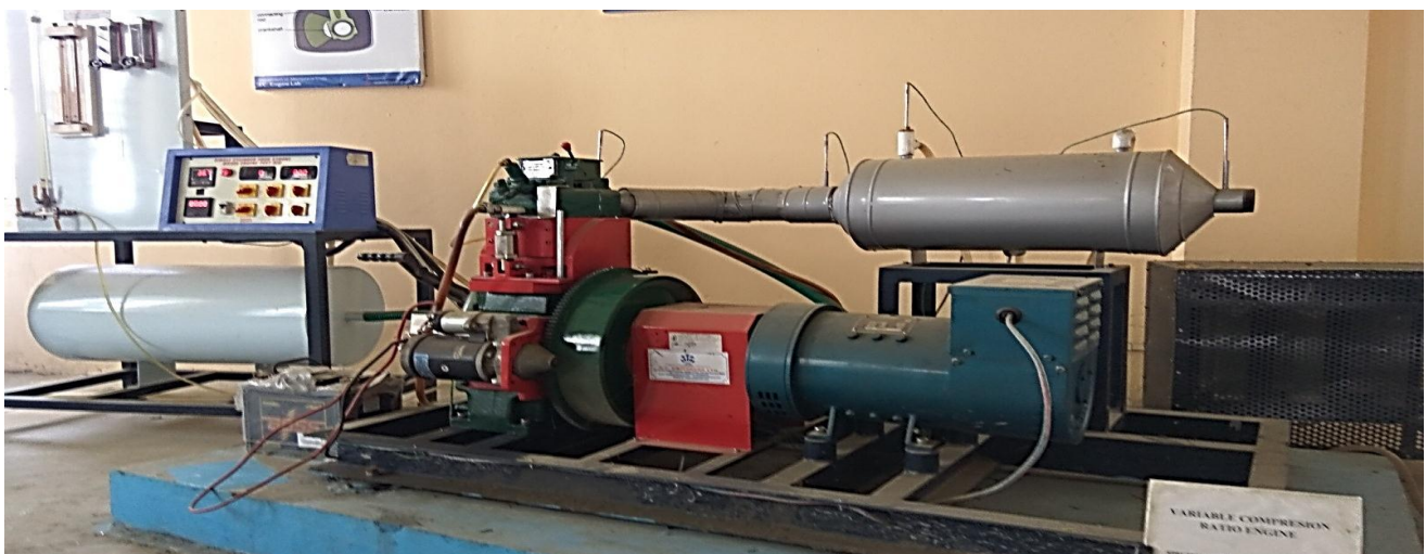
Figure 1.2 – Experimental setup and test rig of Variable Compression Engine
