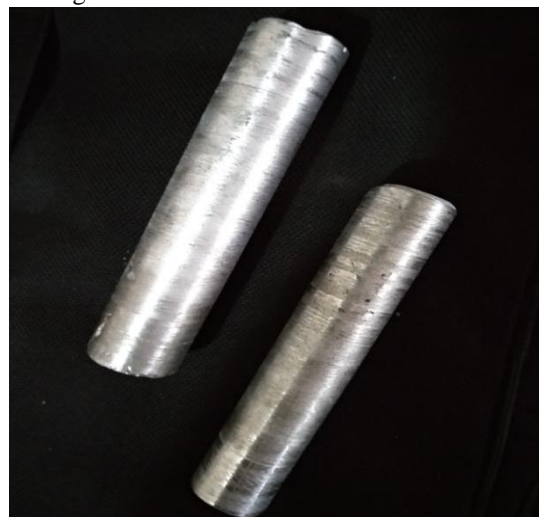
Fig. 6. The two castings after being turned to accurate dimensions of 14 mm diameter.
