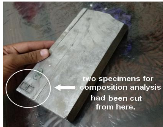
Fig.2. We took two square prisms from the aluminum 6061 alloy piece in order to carry out spectrometry analysis.
