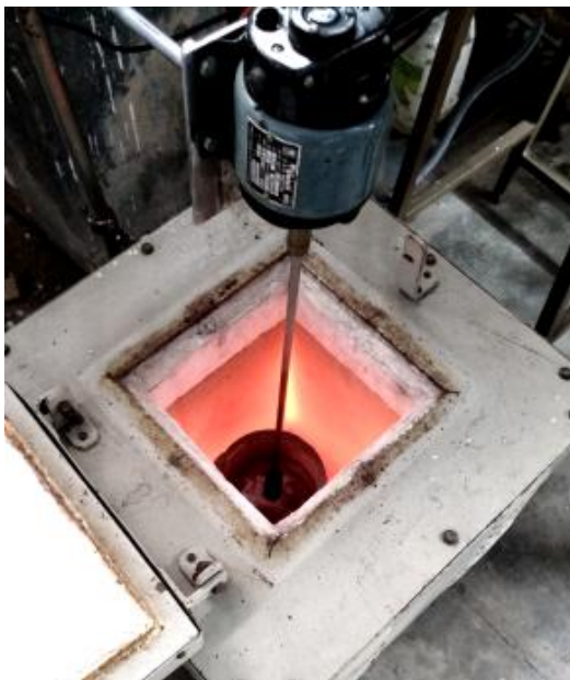
Fig. 4. A stirrer of graphite was used by us to rotate the liquefied contents of the crucible placed in the furnace. We then poured the molten metal into two specially prepared cylinder molds. These cylindrical molds were made of metal and were embedded in casting sand, as shown in Figure 5.
