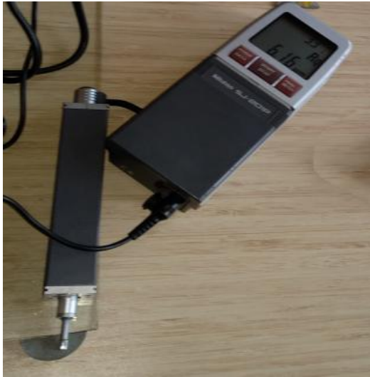
Fig. 10. Photograph of the roughness testing of one of the semi circular shaped pieces being carried out.
