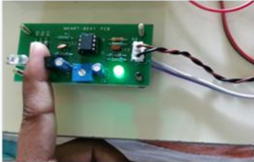
Fig 4. Heartbeat calculation by placing the finger
