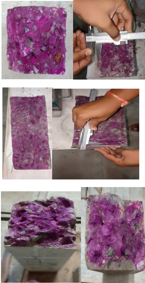
Fig 12. Phenolphthalein test for water cured and CO 2 cured specimens
