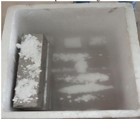
Fig 2. Specimens cured in Dry ice
