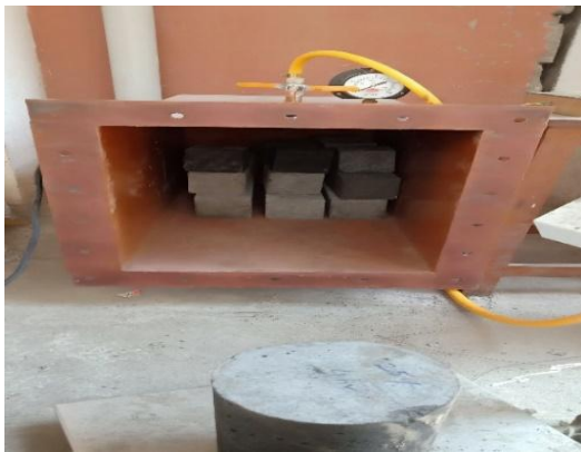
Fig 2. Specimens cured in Dry ice
