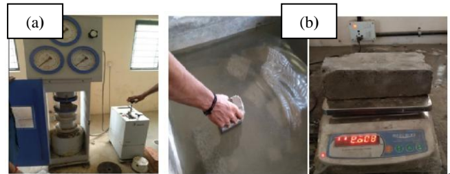
Fig. 4: a) Compressive strength testing machine b) Immersion of brick in water c) Water absorption test
