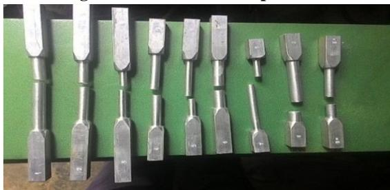
Fig. 2: Specimens after Torsion
