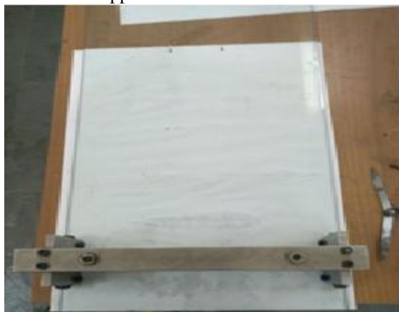
Fig. 2 Membrane casting using casting knife on smooth surface glass
