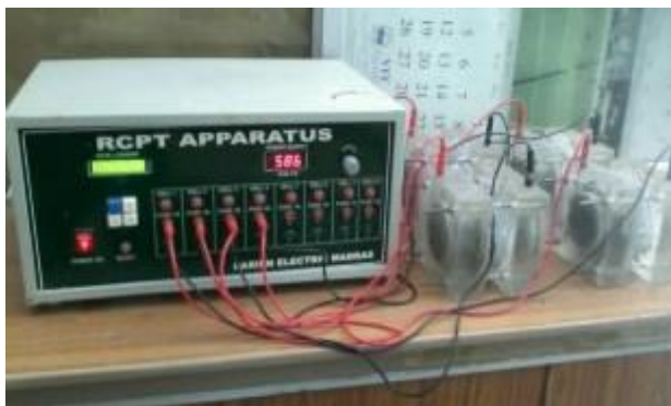
Fig. 7. Image for rapid chloride permeability
