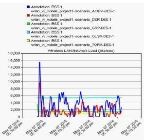
Fig. 17 Network Load of Wireless LAN in BSS1 (As is)
