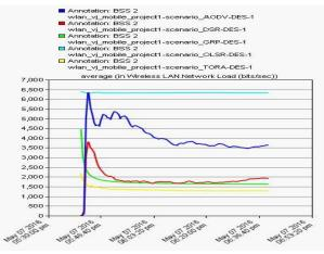
Fig. 20 Average Network Load of Wireless LAN in BSS2
