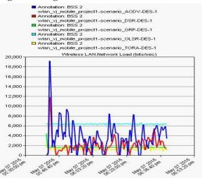
Fig. 19 Network Load of Wireless LAN in BSS2 (As is)
