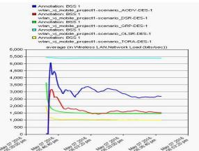
Fig. 18 Average Wireless LAN Network Load BSS1
