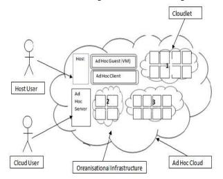
Fig .4 Architecture of the ad hoc cloud [1]
