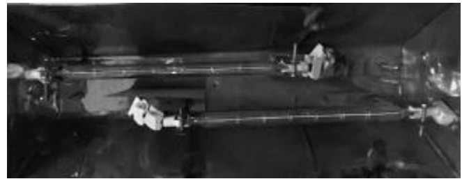
Fig 3. Arrangement of short wave IR heater lamp
