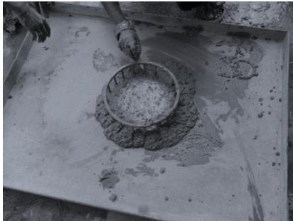
Figure 7 J-ring test on SCC trial mix
