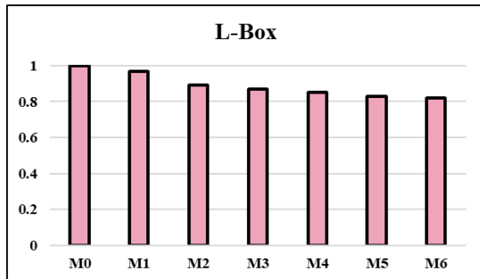
Figure 9 L-Box test of SCC mix
