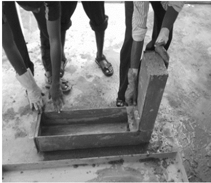
Figure 6 L-box test on SCC
