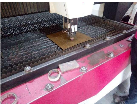
Figure (1): A Picture of a Fibre Laser Beam Machine working on Architectural Brass Plate.
