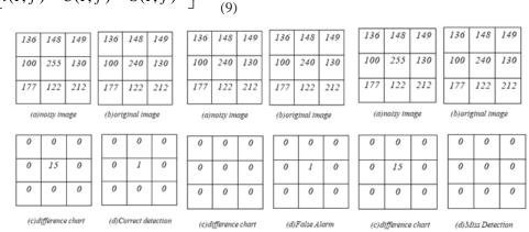
figure4: Difference based method for FA and MD
