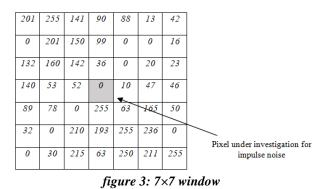
A 7×7 window is used for demonstration of work instead of  $21 \times 21$  window for the first impulse noise detection phase for a crisp view. FCM classify the adjacent 49 pixels unsupervisely in three clusters let Q, R and S.
