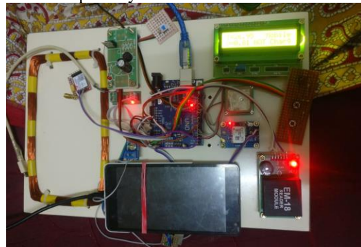
Fig.9. Hardware image of Secondary side of the wireless module and receiver part with mobile battery
