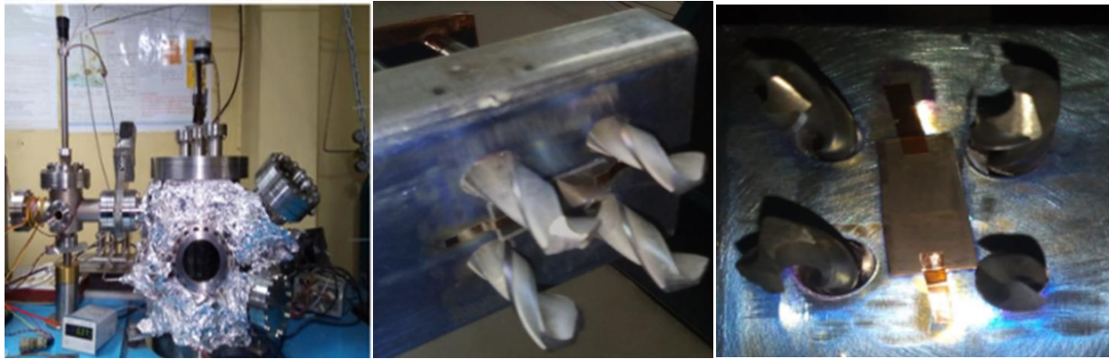
Figure 1. Reactive DC Magnetron Sputtering vacuum chamber, loaded HSS drill bits and deposition
