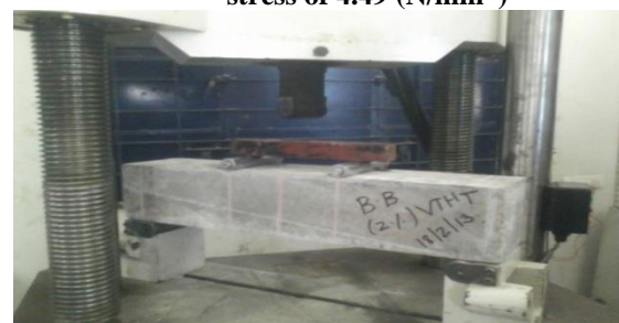
Fig (Q) Failure of 2% CFRC specimen having stress of 4.28 (N/mm 2 )
