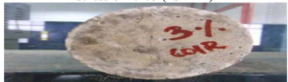
Failure of 3% CFRC specimen having stress of 5.89 (N/mm 2 )
