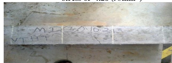
Fig (R) Failure of 3% CFRC specimen having stress of 5.29 (N/mm 2 )
