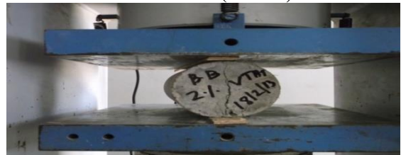
Fig (X) Failure of 2% CFRC specimen having stress of 3.72 (N/mm 2 )
