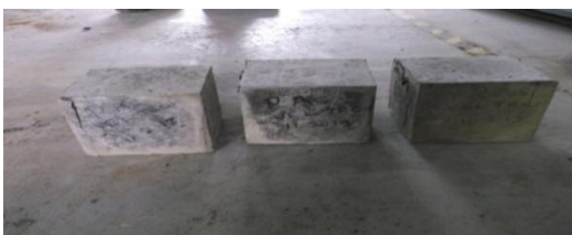
Fig 7(G) Failure of control specimen having stress of 52.99 (N/mm 2 )
