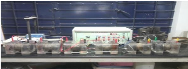
Fig (Z) Exerimental Set Up Of Rcpt
