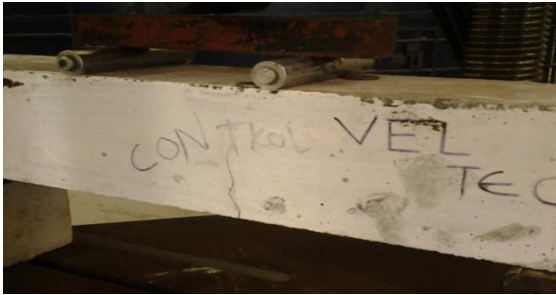
Fig (S) Failure of control specimen having stress of 5.51 (N/mm 2 )
