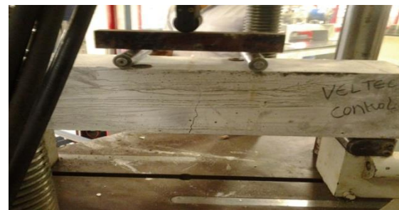
Fig (P) Failure of control specimen having stress of 4.49 (N/mm 2 )
