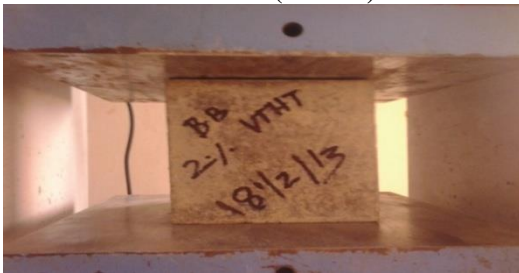
Fig (E) Failure of 2%CFRC specimen having stress of 42.84 (N/mm 2 )
