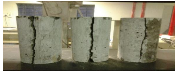
Fig 2(W) Failure of control specimen having stress of 3.82 (N/mm 2 )
