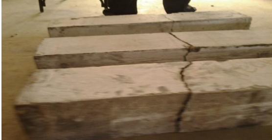
Fig (T) Failure of 2% CFRC specimen having stress of 4.93 (N/mm 2 )
