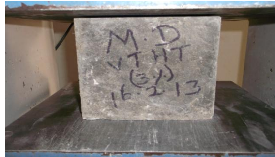
Fig (I) Failure of 3% CFRC specimen having stress of 54.86 (N/mm 2 )
