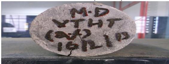
Failure of 2% CFRC specimen having stress of 4.103 (N/mm 2 )
