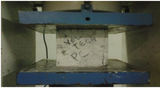
Fig(D) Failure of control specimen having stress of 46.40 (N/mm 2 )
