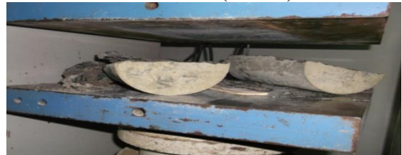
Fig (Y) Failure of control specimen having stress of 4.16 (N/mm 2 )
