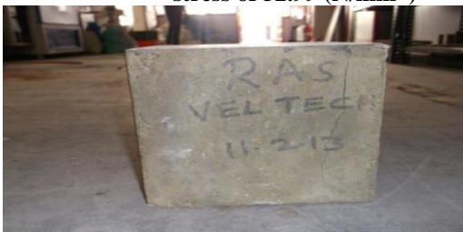
Fig 8(H) Failure of 2% CFRC specimen having stress of 47.62 (N/mm 2 )
