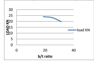
The graphs are plotted between b/t ratio and ultimate load obtained from the experiment for various load positions
