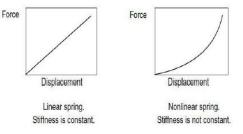
Figure 1: linear and nonlinear spring characteristics
