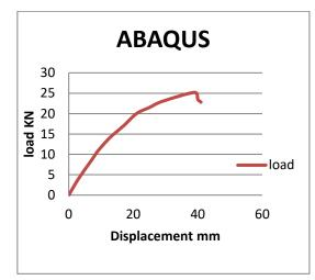
Graph 4: Load vs. Displacement for column 1
