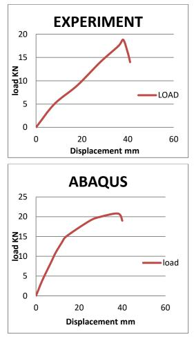
Graph 12: Load vs. Displacement for column 9
