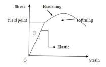
Figure 3: Strain Hardening behaviour
