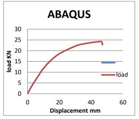
Graph 6: Load vs. Displacement for column 3
