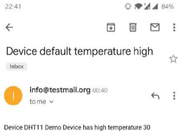
Fig. 6 b) Email received when alarm is triggered
