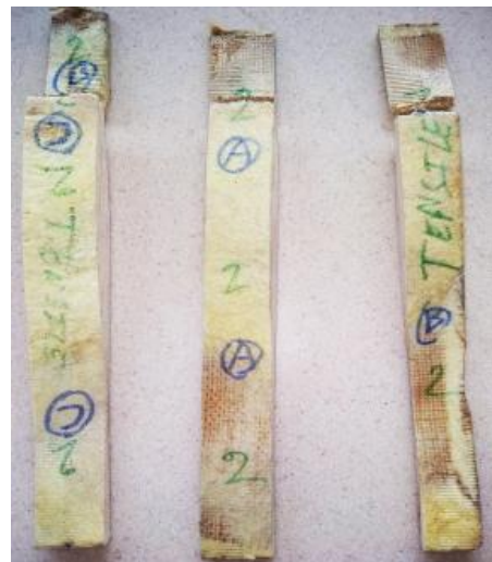
Fig. (7) Fractured specimens when subjected to Tensile test
