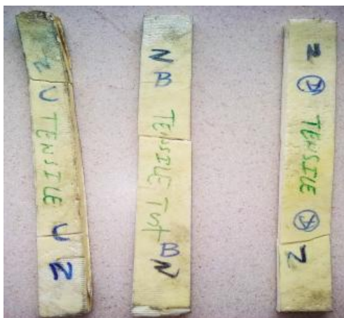
Fig. (9) Fractured specimens when subjected to Tensile test
