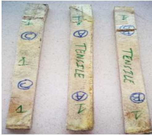
Fig. (5) Fractured specimens when subjected to Tensile test
