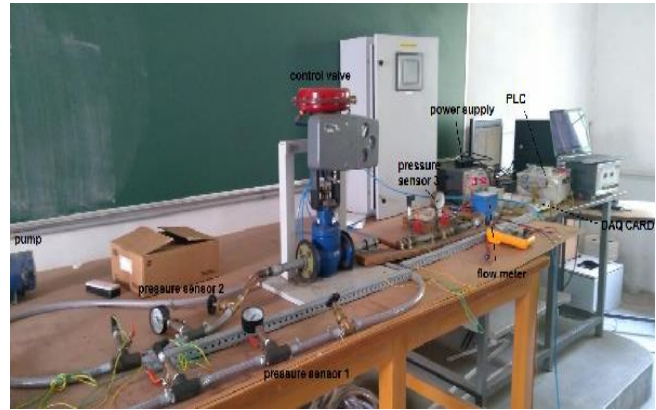
Figure 3. Lab Scale Experimental Set Up Of Oil Pipeline Transport System
