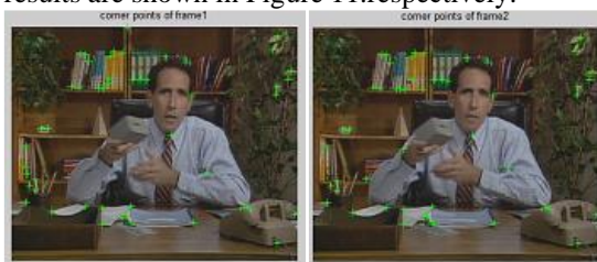
Figure 8: (a) Detection of corner points of frame1. (b) Corner points of frame2 (using KLT)
