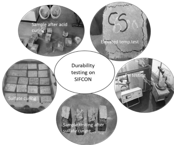
Figure 11. Durability testing on SIFCON
