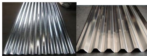
(b) Sine wave Roughness (c) Trapezoidal Roughness
